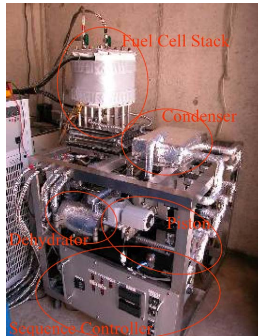
Fig. 6. Fuel cell system combining PEFC stack, gas circulator, and dehydrator.
